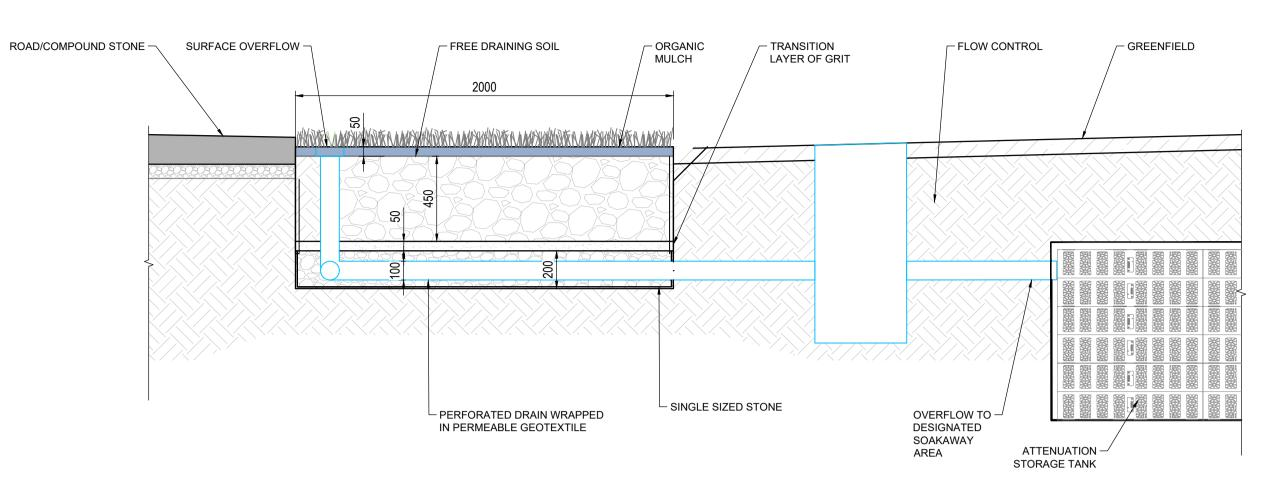
TYPICAL BIORETENTION RAIN GARDEN DETAIL FOR ROADS
