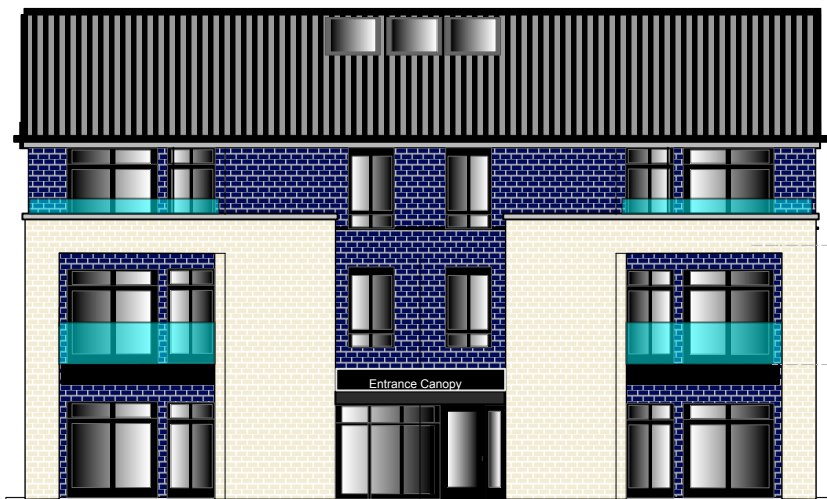
North Elevation Scale 1:100
